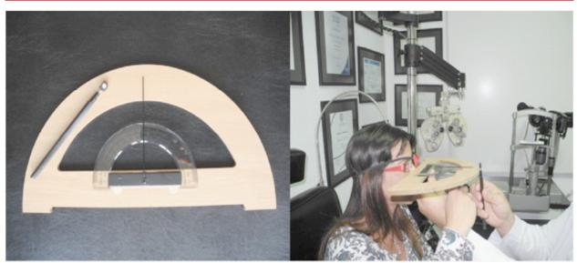
**Fig1.** Pointer perimeter device consisting in a protractor fitted with a bar, thus enabling the experimenter to measure precision in the task of locating target points placed in different directions in the visual field.
